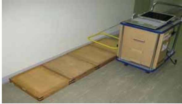
Figure 4 Read experiment by shielding material(wood)
