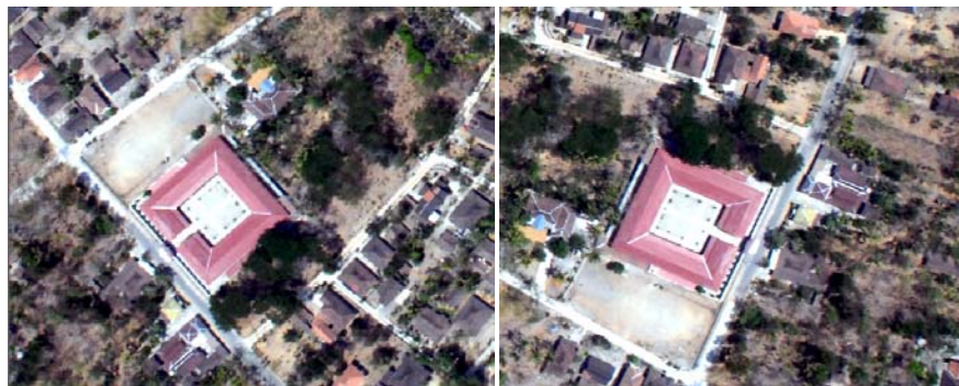
Figure 5. Sample of uncorrected photo (left) and semi-orthophoto extracted (right)
