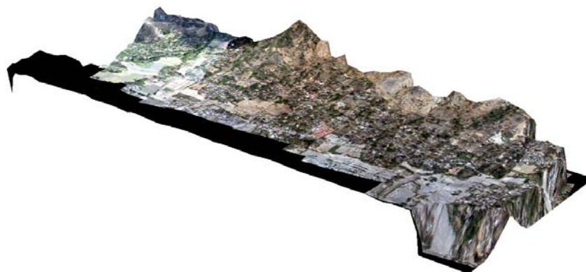
Figure 8. Overlay semi-orthophoto mosaic on DTM data
